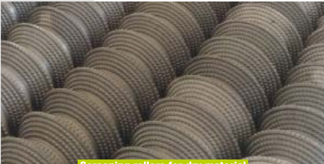
Screening rollers for dry material
